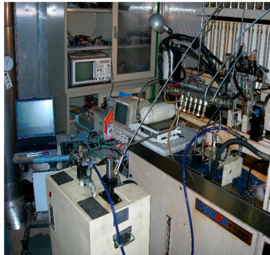
**Figure 1.** Photograph of common rail injection system and test bench.
