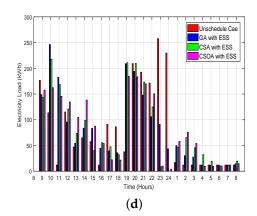
**Figure 8.** Hourly electricity consumption for single and multiple homes. (a) Hourly electricity load for a single smart home without ESS; (b) hourly electricity load for 30 smart homes without ESS; (c) hourly electricity load with ESS for a single smart home; (d) hourly electricity load with ESS for 30 smart homes.
