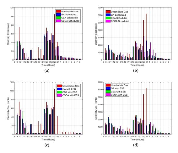
**Figure 9.** Hourly electricity cost using RTP signals. (a) Hourly electricity cost for a single smart home without ESS; (b) hourly electricity cost for 30 smart homes without ESS; (c) hourly electricity cost with ESS for a single smart home; (d) hourly electricity cost with ESS for 30 smart homes.
