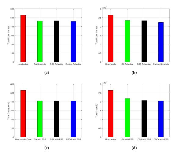
**Figure 10.** Total electricity cost using RTP signals. (a) Total electricity cost for a single smart home without ESS; (b) total electricity cost for 30 smart homes without ESS; (c) total electricity cost with ESS for a single smart home; (d) total electricity cost with ESS for 30 smart homes.
