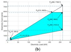
**Figure 4.** Feasible region for cost and electricity consumption using RTP. (a) Feasible region for a single home; (b) feasible region for multiple homes.
