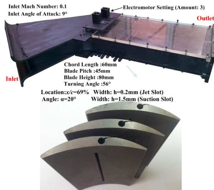
Figure 20. Experimental system and blades with slots.
