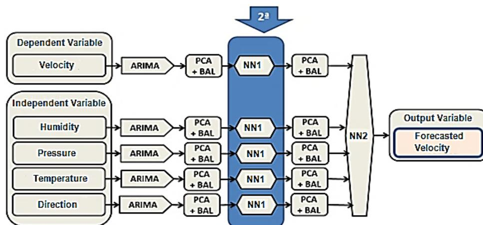
Figure 4. Block diagram of the second stage of the model—ARIMA + NN1.
