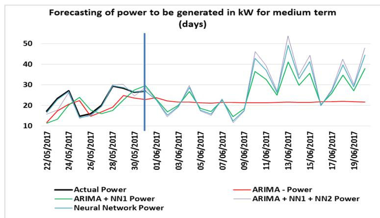
Figure 13. Power Generation Predicted for medium term (days) in kW.
