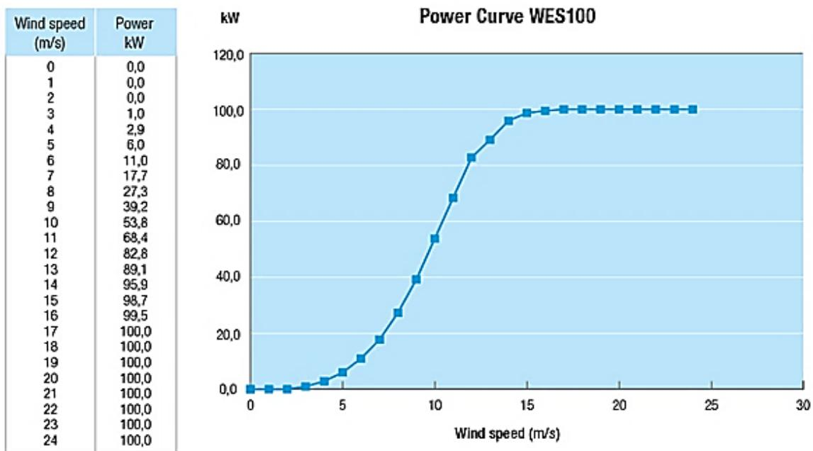
Figure 6. Power curve of the WES100 wind turbine. Source: <http://www.energiapura.com/aerogerador-wes-100>.
