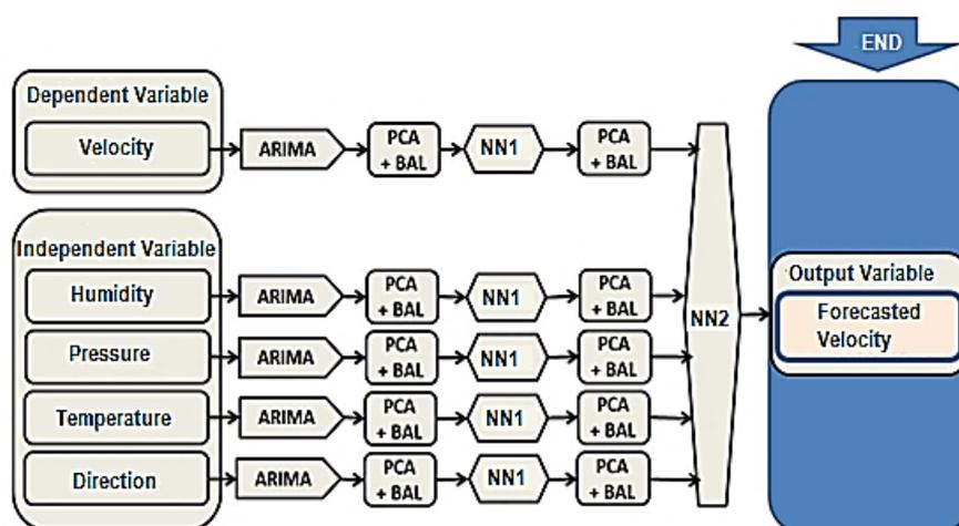
Figure 5. Block diagram of the final step of the model—ARIMA + NN1 + NN2.
