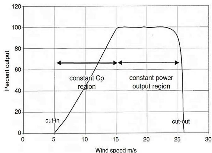
**Figure 1.** Regions of turbine speed control. Source: [11].
