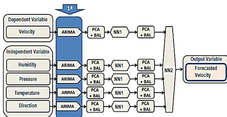
Figure 3. Block diagram of the first stage of the model—ARIMA.
