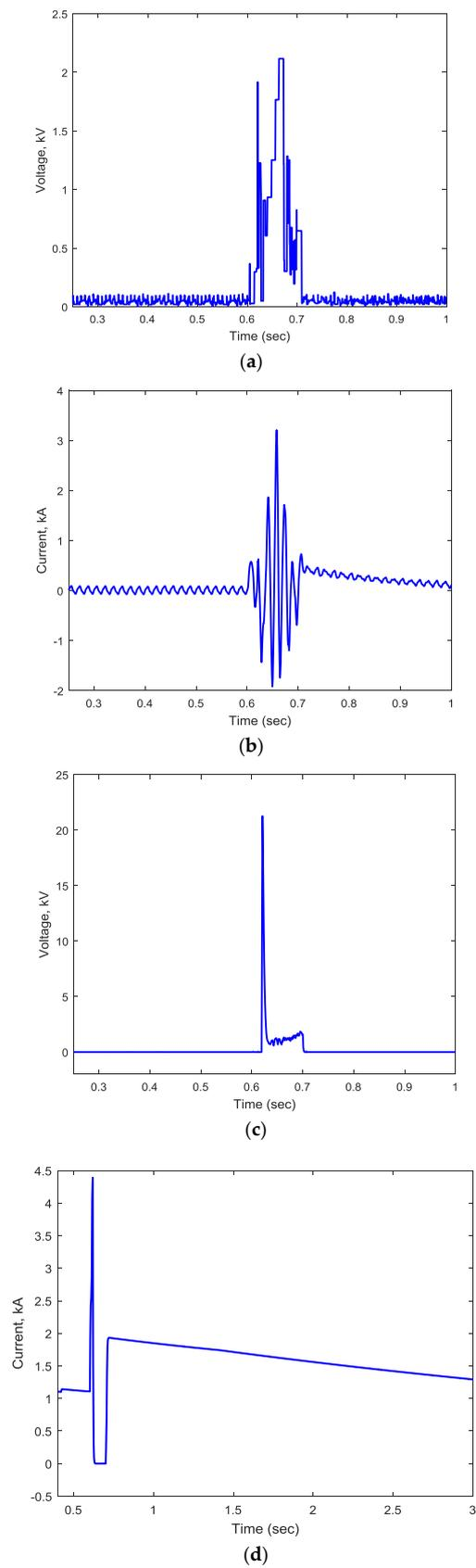
**Figure 6.** Voltage and current stresses of BFCL subject to symmetrical fault at grid1 (a) Voltage across shunt branch (b) Current through the shunt branch (c) Voltage across IGBT switch (d) Current through IGBT switch.
