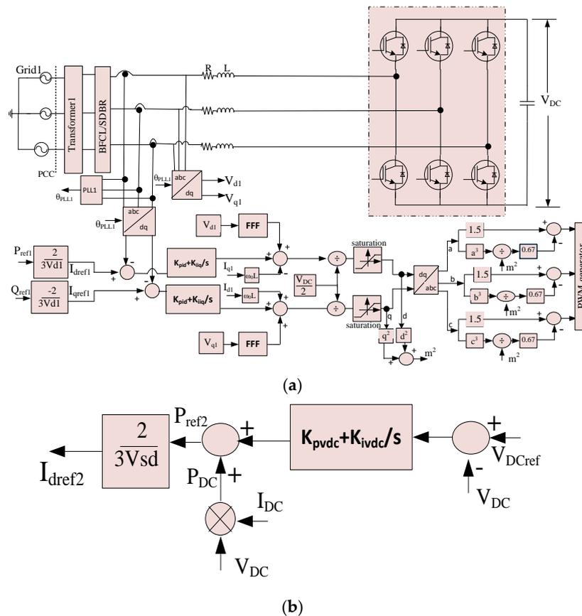
**Figure 3.** HVDC system controllers (a) VSC1 controller with BFCL/SDBR (b) VSC2 controller with BFCL/SDBR.
