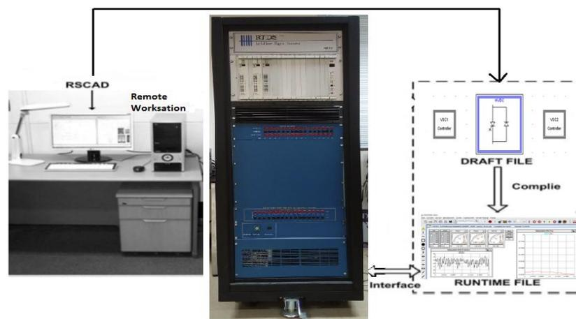
**Figure 4.** Real Time Digital Simulator setup.
