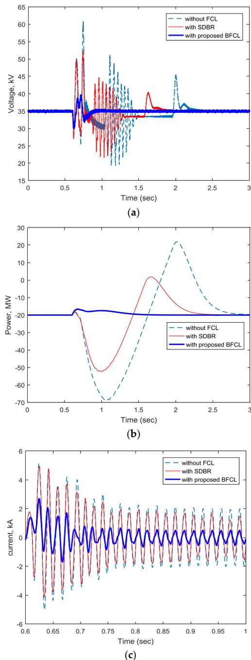
**Figure 5.** Comparative transient response of two grids connected VSC-HVDC system subject to symmetrical fault at grid1 (a) DC link voltage (b) Grid1 active power flow (c) Phase 'a' current of grid1.
