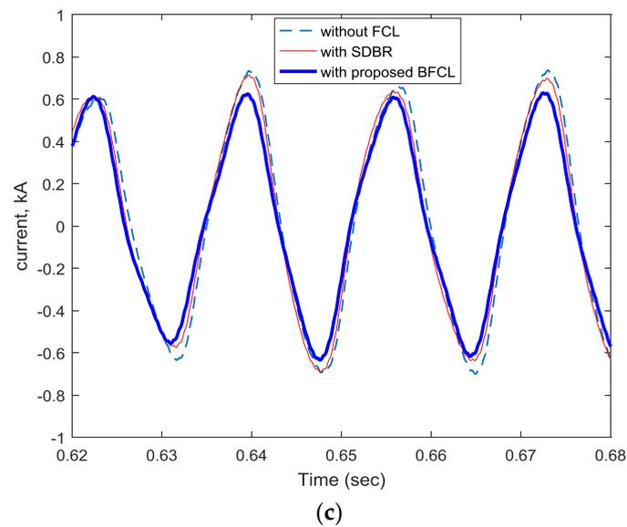
**Figure 8.** Comparative transient response of a two grids-connected VSC-HVDC system subject to a 1LG fault at grid1 (a) DC link voltage (b) Grid1 active power flow (c) Phase 'a' current of grid1.
