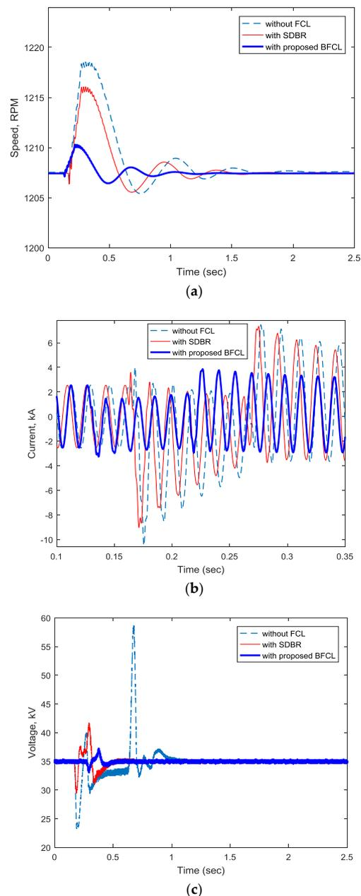
**Figure 7.** Comparative transient response of fixed speed wind integrated VSC-HVDC system subject to symmetrical fault at PCC (a) Induction machine speed (b) Induction machine stator current (c) DC link voltage.
