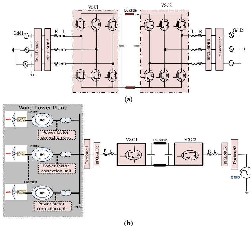
**Figure 2.** Schematic diagram of VSC-HVDC systems (a) Two grids connected mode (b) Wind farm integrated mode.
