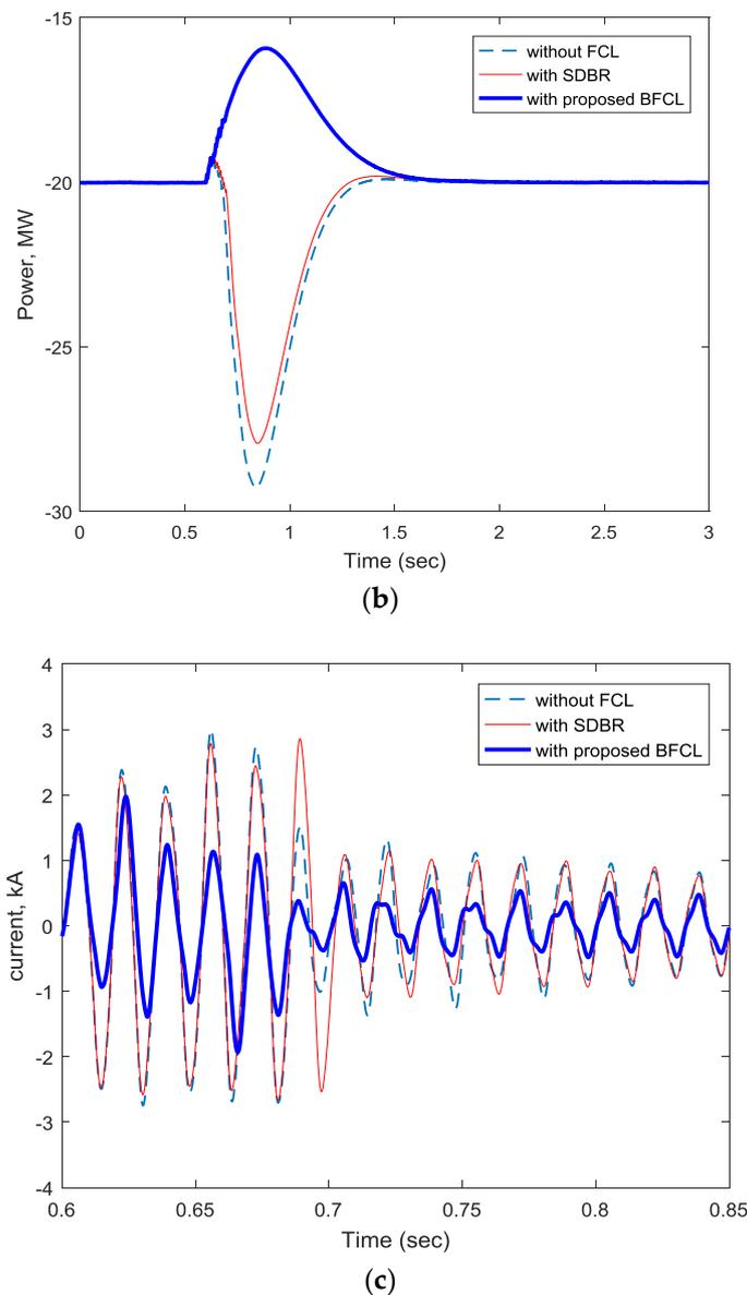
**Figure 9.** Comparative transient response of two grids connected VSC-HVDC system subject to 2LG fault at grid1 (a) DC link voltage (b) Grid1 active power flow (c) Phase ‘a’ current of grid1.
