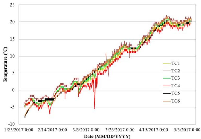
Figure 12. Temperature profile of each sand-bed measurement location.
