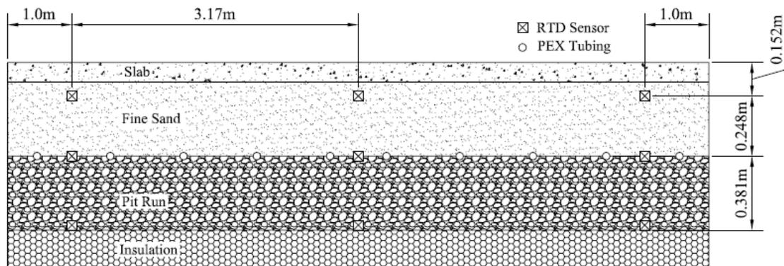
Figure 8. Resistive temperature detectors (RTD) locations in sand-bed.
