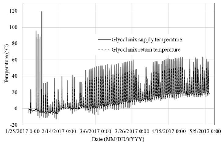
Figure 10. RTD measured glycol supply and return temperatures.
