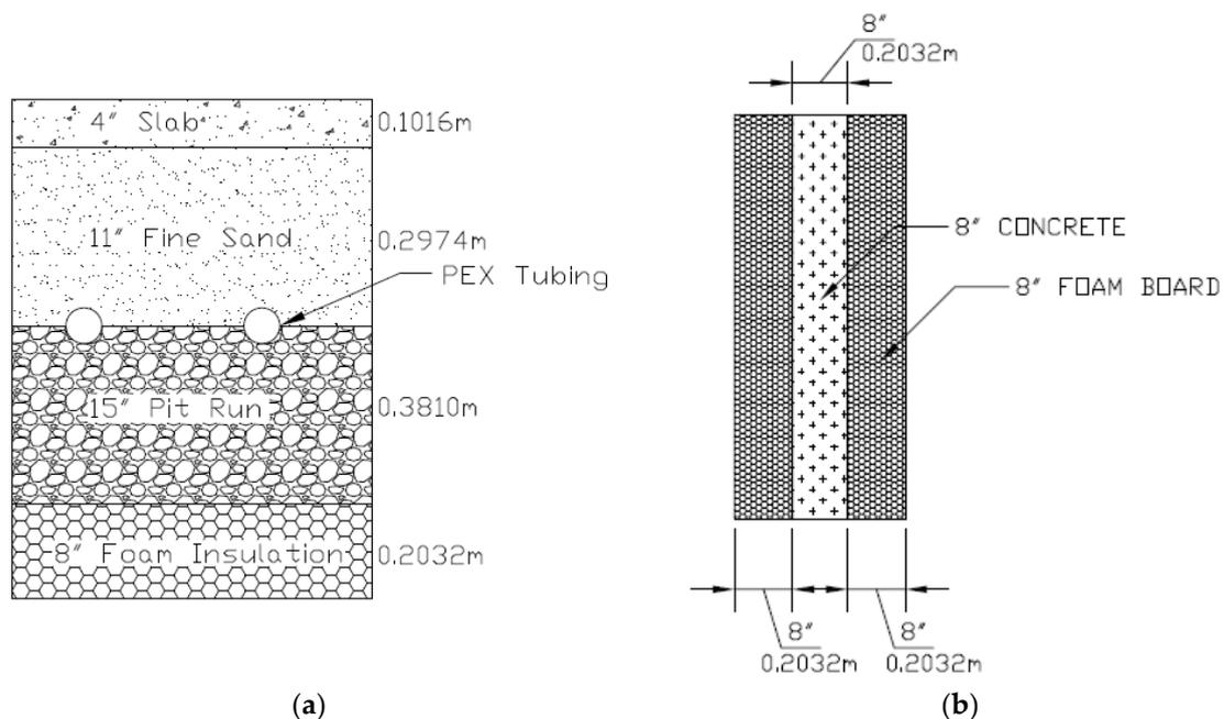
Figure 6. (a) Profile of solar thermal storage; (b) foundation wall cross-section.
