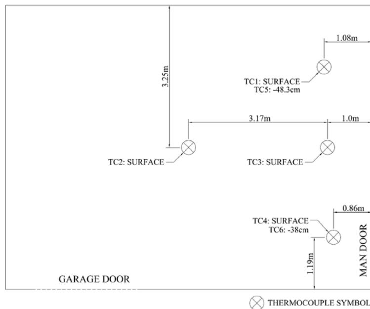
**Figure 9.** Thermocouple arrangement on sand-bed thermal storage.
