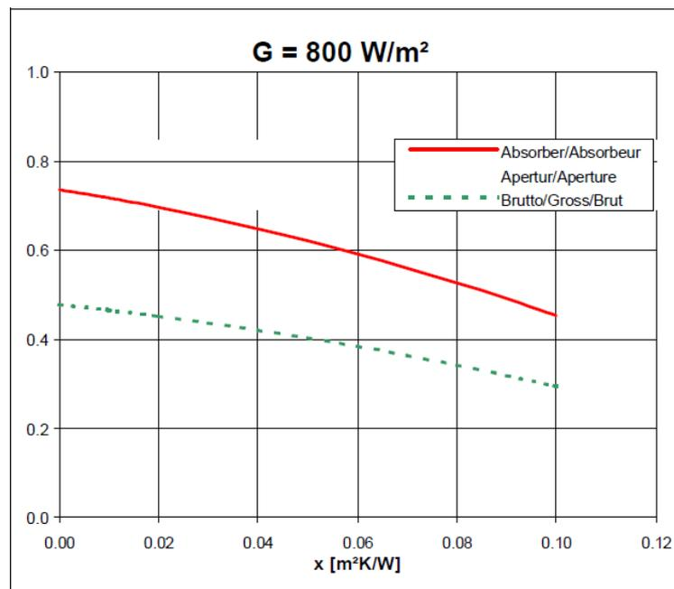
**Figure 2.** Sunda Seido 5-16 efficiency curve, image from Solartechnik [16].
