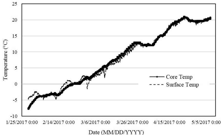
**Figure 13.** Average sand-bed core temperature and surface temperature.
