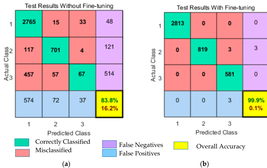
Figure 11. Performance of fine-tuning strategy is displayed with confusion matrix: (a) Results without fine-tuning; (b) Results with the fine-tuning approach.
