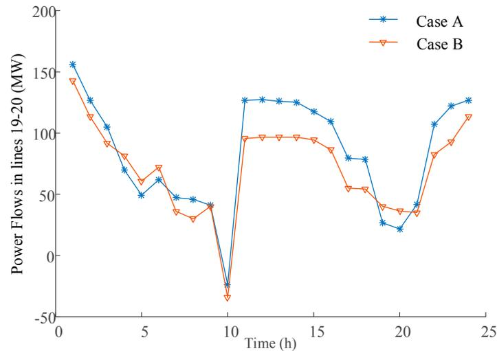
Figure 9. Power flows in line 19–20 in day-ahead scheduling stage.
