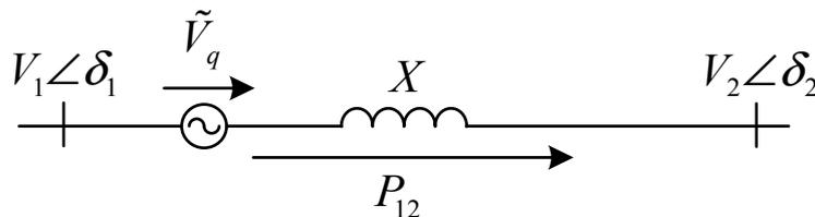
Figure 4. Circuit model of a transmission line with DPFC.
