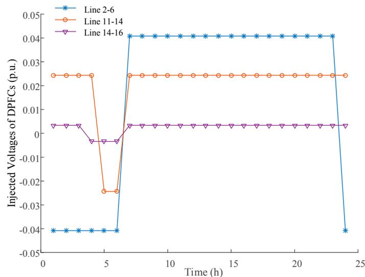
**Figure 11.** Optimal control strategy of DPFCs in real-time scheduling stage.
