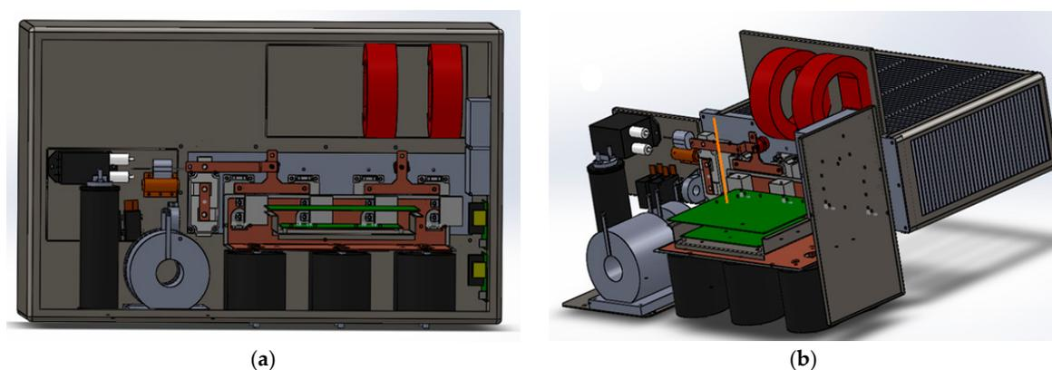
**Figure 2.** Electro-mechanical concept diagram of DPFC. (a) Front view of DPFC, and (b) Lateral view of DPFC.
