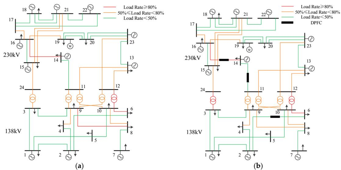
Figure 6. Power flows in IEEE-RTS79 system, (a) without DPFCs, and (b) with DPFCs.
