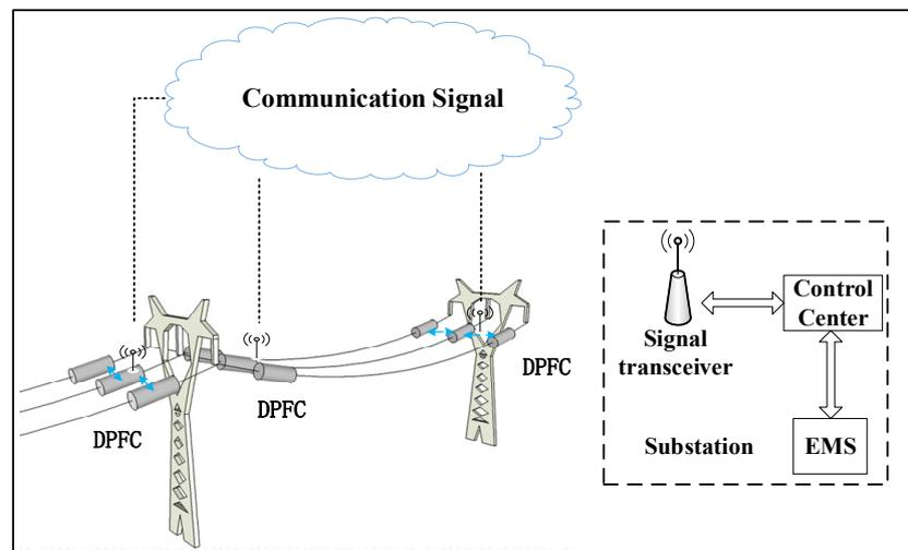
**Figure 1.** Distributed power flow controller (DPFC) deployed on transmission line.
