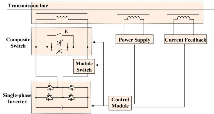
Figure 3. Schematic representation of a DPFC.
