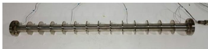
Figure 5. Photograph of the fabricated annular finned tube.
