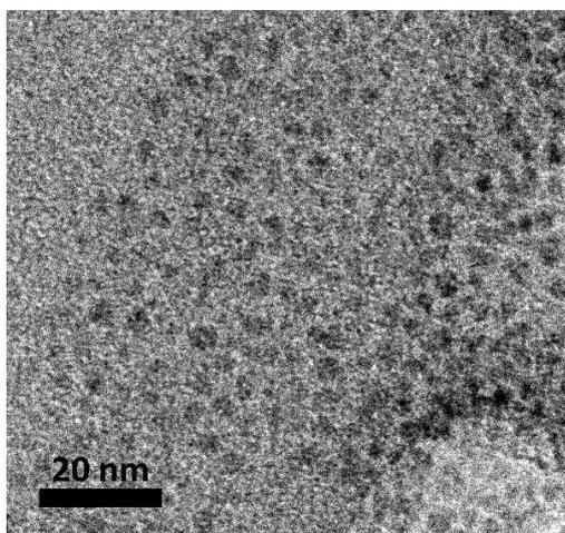
Figure 1. (b) TEM picture for carbon dots at ~5 nm.
