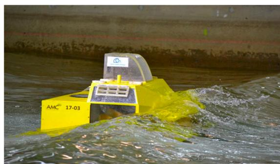
**Figure 2.** Model scale experiments performed in the Australian Maritime College's Model Test Basin [7].
