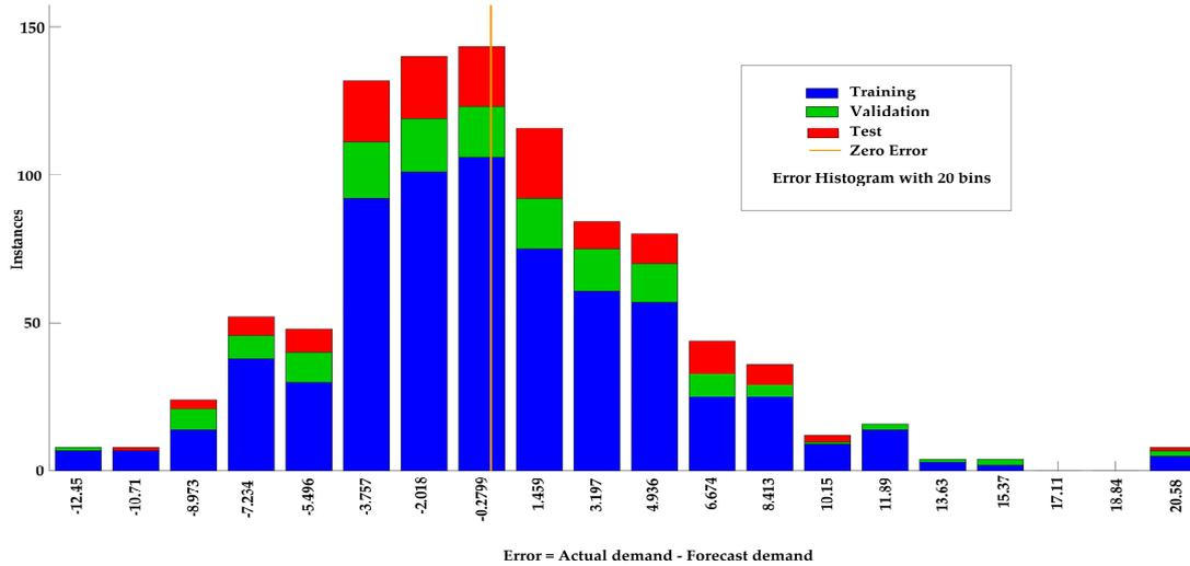
**Figure 9.** Illustration of the forecast error for training, validation and testing data in a histogram, where 70% of the historical data has been used as training, 13% as validation data and 17% as testing data (5 days testing).
