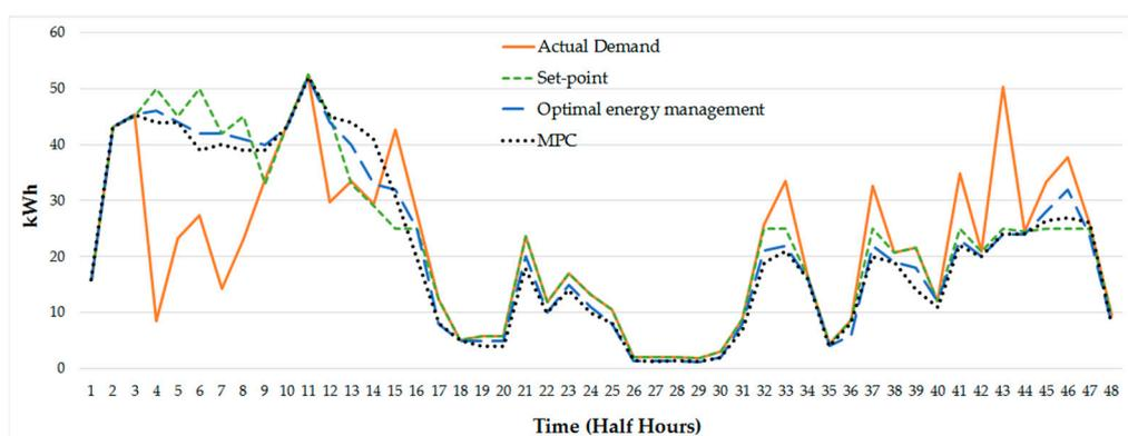
**Figure 11.** Specific example results: The actual demand, optimal energy management controller results and MPC controller results for one day.
