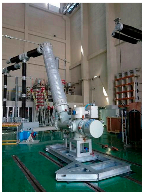
Figure 8. The 420 kV 63 kA HSES model.
