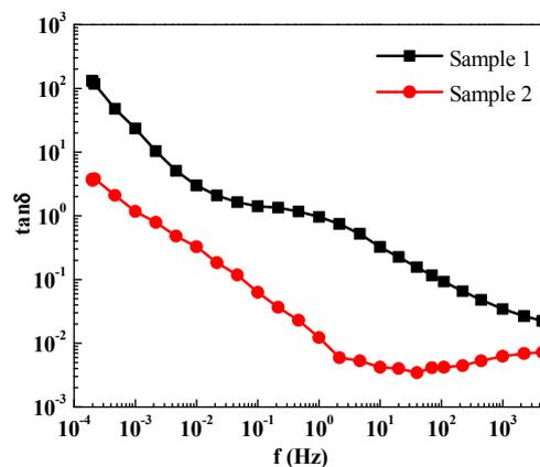
Figure 5. FDS results of Sample 1 and Sample 2.
