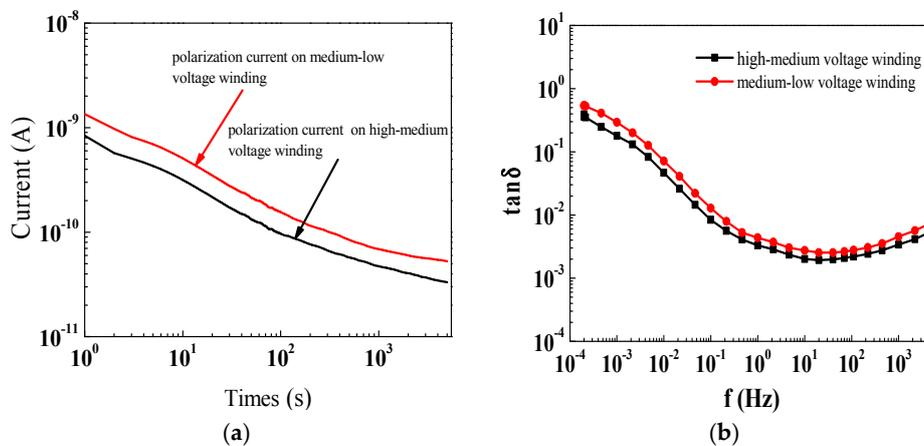
Figure 8. The time and frequency domain spectroscopy of the transformer cellulose insulation. (a) polarization current; (b)  $\tan \delta$ .
