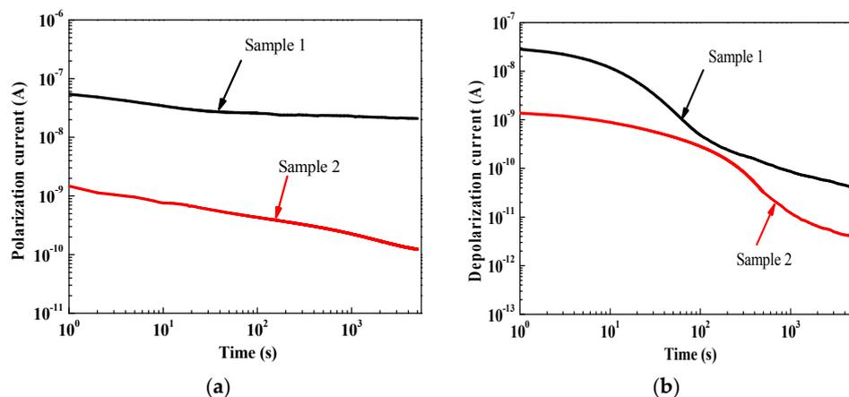
Figure 4. Polarization and depolarization current results of (a) Sample 1 and (b) Sample 2.
