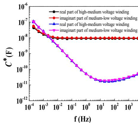
Figure 7. The  $\epsilon^*_{tot}(\omega)$  spectroscopy of the transformer main insulation.
