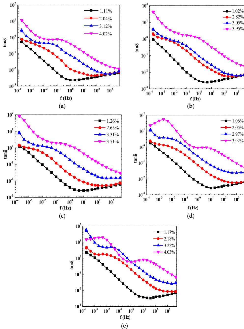
**Figure 3.** FDS results of oil-impregnated pressboards. (a) Aged 0 day; (b) Aged 8 days; (c) Aged 21 days; (d) Aged 32 days; and (e) Aged 42 days.
