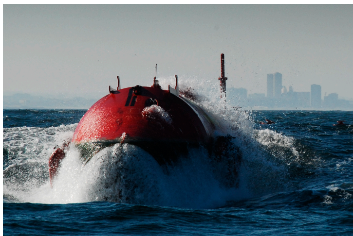
Figure 2. The Pelamis wave energy converter. (Source: Pelamis Wave Energy Converter on site at the European Marine Energy Test Center (EMEC) by P123, retrieved from https://commons.wikimedia.org/wiki/File:Pelamis_at_EMEC.jpg ).
