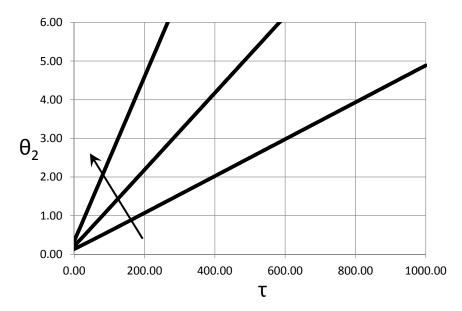
**Figure 3.** Dynamics of the smoke (upper layer) temperature in non-dimensional variables. The arrow points towards an increase of the non-dimensional heat release rate for each of the curves:  $\dot{Q} = 4.55 \times 10^{-3}$ ;  $\dot{Q} = 9.10 \times 10^{-3}$  and  $\dot{Q} = 1.82 \times 10^{-2}$ .
