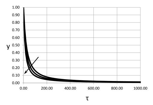
**Figure 2.** Dynamics of the smoke layer interface in non-dimensional variables. The arrow points towards an increase of the non-dimensional heat release rate for each of the curves:  $\dot{Q} = 4.55 \times 10^{-3}$ ;  $\dot{Q} = 9.10 \times 10^{-3}$  and  $\dot{Q} = 1.82 \times 10^{-2}$ .
