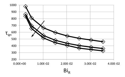
**Figure 5.** Influence of the radiation Biot number on ignition time. Both variables are non-dimensional. The arrow points towards an increase of the parameter E for each of the curves:  $E = 3.79 \times 10^5$ ;  $E = 1.14 \times 10^6$  and  $E = 1.90 \times 10^6$ .
