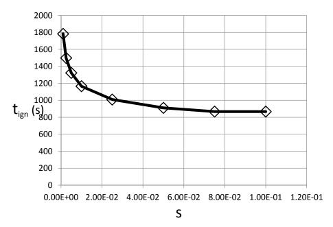
**Figure 8.** Dependence of the dimensional ignition time on the non-dimensional fuel soot yield.  $\widetilde{H} = 3$  m;  $\widetilde{S} = 16$  m<sup>2</sup>.
