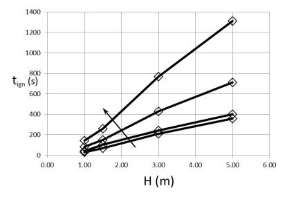
**Figure 9.** Influence of the height clearance on the dimensional ignition time. The arrow points towards an increase of the fuel area S for each of the curves:  $S = 12 \,\text{m}^2$ ;  $S = 24 \,\text{m}^2$ ;  $S = 48 \,\text{m}^2$  and  $S = 100 \,\text{m}^2$ .
