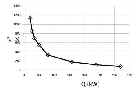
**Figure 7.** Dimensional ignition time as a function of the dimensional initial fire HRR.  $\widetilde{H}=3\,\mathrm{m}$ ;  $\widetilde{S}=16\,\mathrm{m}^2$ .
