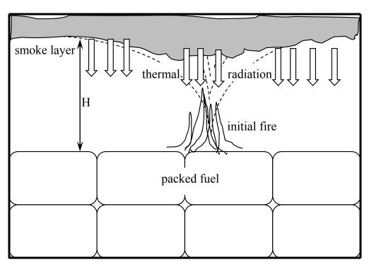
Figure 1. Flashover development scenario in a cargo compartment of a ship.
