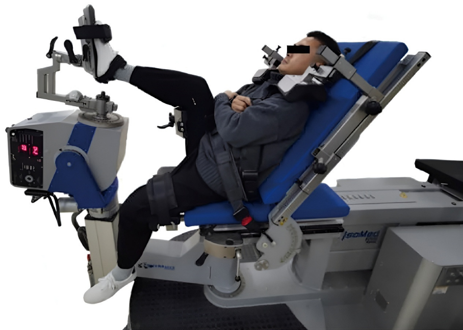
Figure 1. Ankle strength and stability testing setup. Positioning of participants on the IsoMed2000 dynamometer and pressure plate system (D&R Ferstl GmbH, Hemau, Germany, and Zebris Medical GmbH, Isny, Germany, respectively), ensuring ankle joint alignment with the rotational axis during dorsiflexion and plantar flexion strength assessments.
