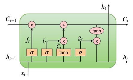
Figure 1. Structure of an LSTM unit.
