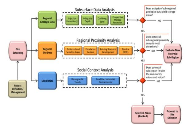
Figure 4. Process flow chart for site screening and initial characterization.
