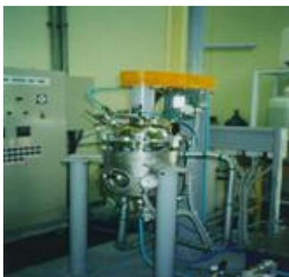
(b) Main reactor for PCC manufacture
