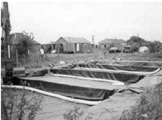
**Figure 10.** Accelerated carbonation treatment equipment (from Jiangying *et al.* [38] with permission of Elsevier).
