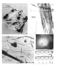
**Figure 1:** Chrysotile asbestos nanotubes. (a) Small mineral sample form large mine in Quebec, Canada. (b) TEM image of individual nanotubes, broken fragments, and small aggregated bundles [42]. (c) Magnified TEM image of aggregated chrysotile nanotubes [41]. (d) SAED pattern corresponding to the aggregate in (c) showing streaking of diffraction spots. (e) Curved layer schematic tube sections spaced 7.5 Å. (After De Souza Santos [39]).
