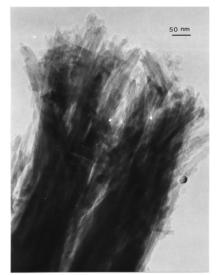
Figure 15: TEM image of MWCNT bundle collected indoors on an electrostatic plate.
