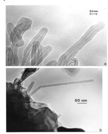
**Figure 13:** TEM images for environmental MWCNTs. (a) MWCNTs collected near a natural gas electric power generation plant. (b) MWCNTs and aggregated graphitic PM in wood soot. (From Murr and Guerrero [50]).
