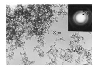
**Figure 18:** Large, fractal-like, branched aggregates of BC created by carbon arc evaporation and observed in the TEM. SAED pattern insert show diffuse graphite reflections.
