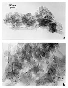
**Figure 12:** Propane flame-derived MWCNT aggregates collected by thermal precipitation and observed in the TEM. (a) Predominantly multiconcentric fullerene nano-PM. (b) Mixture of MWCNTs and multiconcentric, faceted fullerenic polyhedra. (From Murr, et al. [49]).
