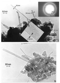
**Figure 9:** TEM images for MWCNT aggregates containing faceted, polyhedral structure. (a) Natural gas (flame) produced. SAED pattern show graphitic reflections noted while the high resolution image insert shows 13 concentric nanotube layers. (b) Propane truck exhaust MWCNT, multiconcentric fullerene aggregate collected by thermal precipitation.
