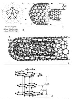
**Figure 7:** Carbon nanotube growth simulations and schematics. (a) Double cap nucleus. (b) Double tube nucleation and growth simulation from (a) forming an armchair tube growing over an armchair tube. ((a) and (b) are from Lair, et al. [44]. (c) Schematic showing a chiral tube growing over the same chiral tube. (d) Ideal graphite lattice and unit cell showing unit cell and graphene lattice dimensions.
