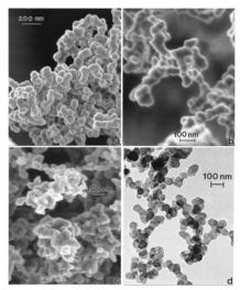
**Figure 16:** FESEM and TEM images of speciated soot PM. (a) FESEM view of candle soot (CPM). (b) Wood soot (WPM) observed in FESEM. (c) Diesel soot (DPM) observed in FESEM. (d) TEM image of tire soot (TPM). (a) to (c) PM collected on glass fiber filters. PM in (d) collected by thermal precipitation. (From Murr, et al [47]).
