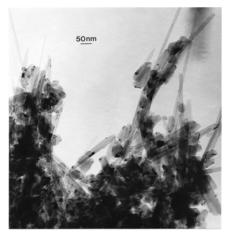
**Figure 3:** TEM image of MWCNT and multiconcentric fullerenes produced by injecting fine tire powder into an electric arc in helium.
