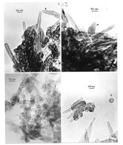
**Figure 10:** TEM image comparison for MWCNT/multiconcentric fullerene PM aggregates collected by thermal precipitation. (a) Pure methane air flame product. (b) Natural gas (96% methane)-air flame product (c) and (d) show propane-air flame products.
