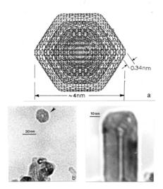
**Figure 11:** Nanostructural faceting of multiconcentric carbon nanoforms. (a) Schematic rendering of 5-layer carbon fullerene or carbon onion (After [48]). (b) Magnified view of carbon nanoform in fig. 10(d) for comparison with (a). (c) Magnified view of MWCNT end cap facets in fig. 9(a).
