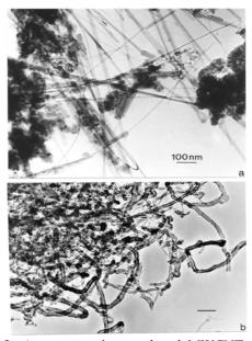
**Figure 2:** Arc evaporation produced MWCNTs (a) and metal catalyst produced MWCNTs (b). (b) is after Soto, et al. [29]. The magnification in (b) is shown in (a).
