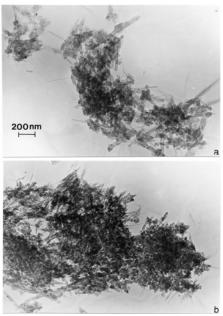
**Figure 4:** TEM bright-field images of MWCNT aggregates collected by thermal precipitation. (a) Variety of MWCNTs and multiconcentric fullerenic PM from propane kitchen range. (b) Dense aggregate of short MWCNTs and multiconcentric fullerenes from outdoor, industrial natural gas source.
