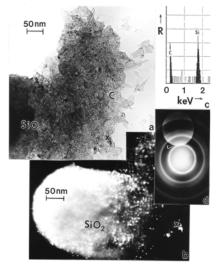
**Figure 14:** Complex aggregate composed of silica  $(SiO_2)$  nano-PM and relatively short MWCNTs and other multiconcentric fullerenes observed in the analytical TEM. (a) Bright-field image. (b) Aperture dark-field image of (a) using the diffraction region marked by arrow in SAED pattern insert in (d). (c) Shows the corresponding EDS spectrum absent the oxygen signal. (From Murr, et al [47]).
