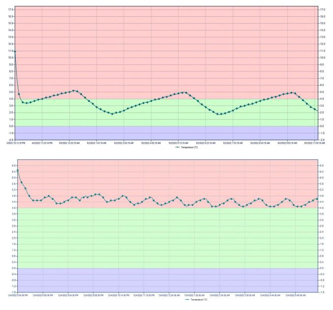
Figure 1. LogTag model TRIX-8 temperature profile of Polish domestic refrigerators.
