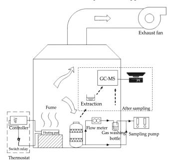
**Figure 1.** Schematic illustration of the experimental apparatus.
