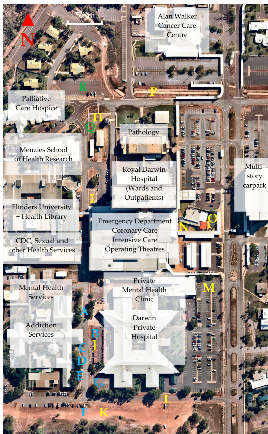
Figure 3. Baseline thermal imaging sites A–G (shown in blue) taken at RDH campus at 3:34 p.m. on 23 August 2021 (temperature 31 °C, relative humidity 56%) and subsequently at sites H–P (shown in yellow) between 3:00 p.m. and 4:14 p.m. on 15 December 2021 (temperature 35 °C, relative humidity 57%). Heat stress measurements (shown in green) were taken at site Q with exposed grass surface and site R with exposed bitumen surface between 3:05 p.m. and 4:05 p.m. on 11 March 2023 (temperature 32 °C, relative humidity 58%).
