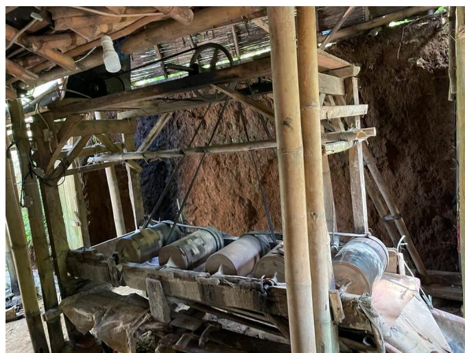
Figure 2. Grinding gold ore with mercury in cylinders. Location: West Java Province.
