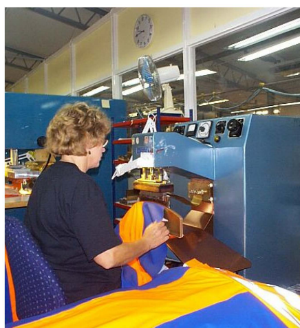
Figure 4. Operator of a plastic welding machine. The exposure of the hands can be quite substantial. The body also gets a rather high exposure. The weld typically lasts for some to a few seconds with a repletion time of some tens of seconds (Hansson Mild, personal communication).
