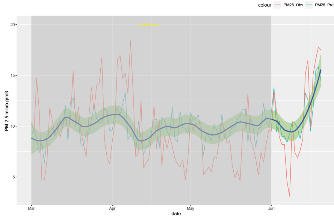
Figure 10. Weather normalized predictions of the pollutant PM 2.5. The blue line represents the smoothed plot of predicted values with the confidence intervals shown by the green shade.
