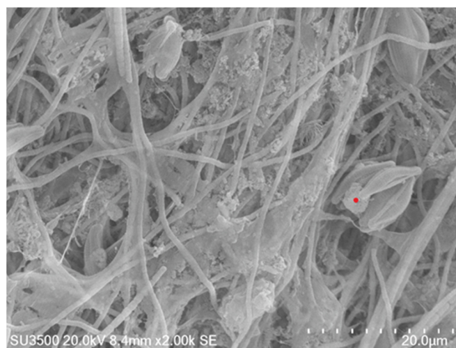
Figure 4. Scanning electron microscope (SEM) microphotograph of algae biofilm showing the formation of mineral phases on the cell surfaces. A typical composition of the inorganic precipitates (given by Energy-dispersive X-ray spectroscopy (EDX) analysis performed on the grain indicted by the red dot) is C ( 40.38\% \pm 4.01 ), O ( 47.2\% \pm 4.13 ), Mg ( 6.27\% \pm 0.21 ), and Si ( 6.15\% \pm 0.17 ), similar to the mineral phase (i.e., \text{MgCO}_3 and \text{SiO}_2 ).
