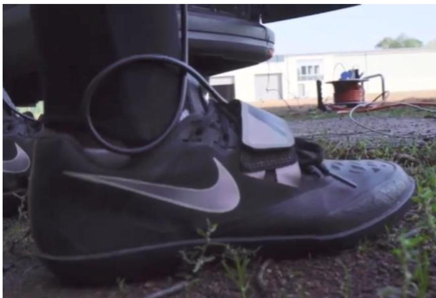
Figure 4. IMU placement under the Velcro fastener of the shoe.
