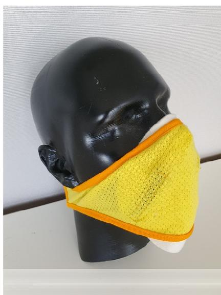
**Figure 2.** Wool–polypropylene fabric filter disc mounted with air permeable wrap to wearer's face.
