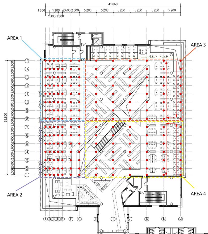
Figure 10. The measuring point layout of A400.
