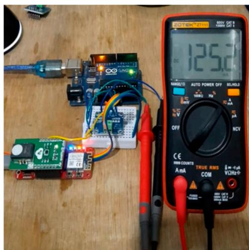
**Figure 9.** Power measurement.
