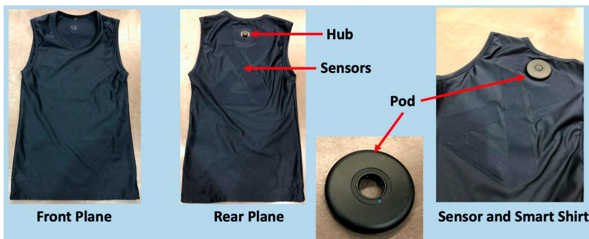
**Figure 2.** External Layout of Tyme Wear Smart Shirt and Pod.
