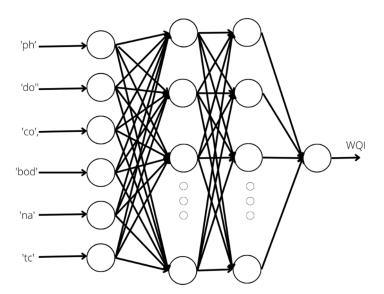
Figure 5. Architecture of the WQI artificial neural network regression (ANN).
