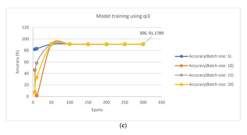
**Figure 9.** Training ANN models using water quality parameters (a)  $qi_1$ , (b)  $qi_2$ , and (c)  $qi_3$ .
