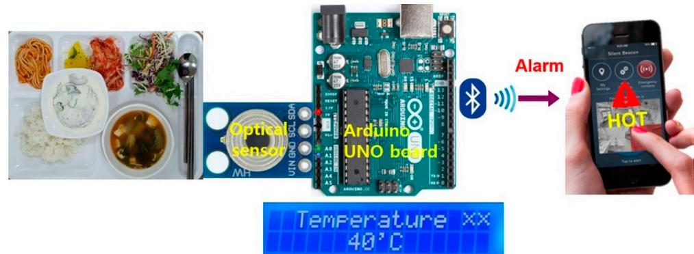
**Figure 4.** Conceptual architecture of a meal temperature-monitoring system.
