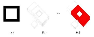
**Figure 8.** Atrial layout. (**a**) Planimetric scheme; (**b**) Axonometric scheme; (**c**) Axonometric scheme with the minimum area that must be dedicated to the infectious disease section indicated red.
