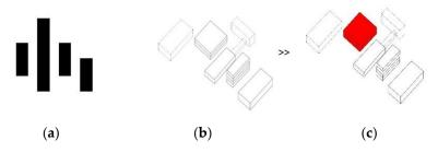
**Figure 2.** Free-standing detached pavilions: cluster/campus layout. (a) Planimetric scheme; (b) Axonometric scheme; (c) Axonometric scheme with the minimum area that must be dedicated to the infectious disease section indicated red.
