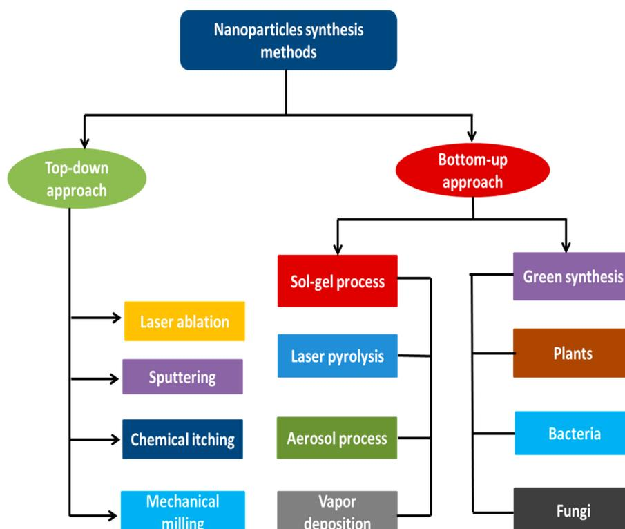
**Figure 1.** Different methods of synthesis of silver nanoparticles using the top-down and bottom-up approaches.
