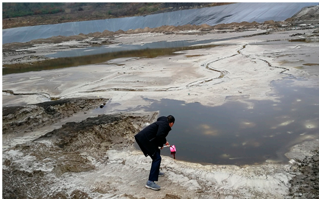
Figure 2. Picture of the sampling of naturally accumulated water from field FGD gypsum dumps (water sample #2).
