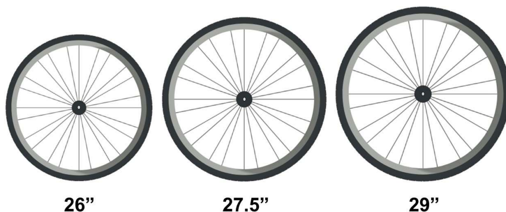
Figure 10. Example of the bike wheel diameters for XC throughout the years.
