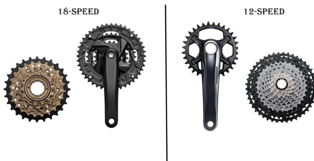
Figure 9. Most popular in the 1990s (18-speed) and more recent (12-speed) gear system models. Although the left system allows more speed combinations, the right one is more accurate, lighter, stronger, more efficient and easier to handle.
