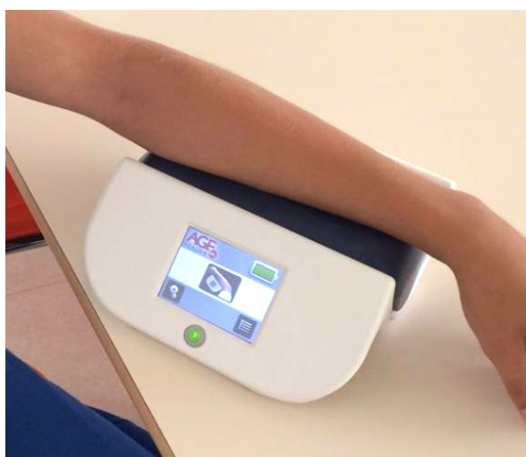
Figure 2. Practical measurement of skin autofluorescence.
