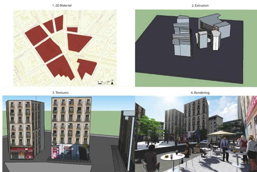
**Figure 2.** 3D modeling procedures (2D Material, Extrusion, Textures, and Rendering).
