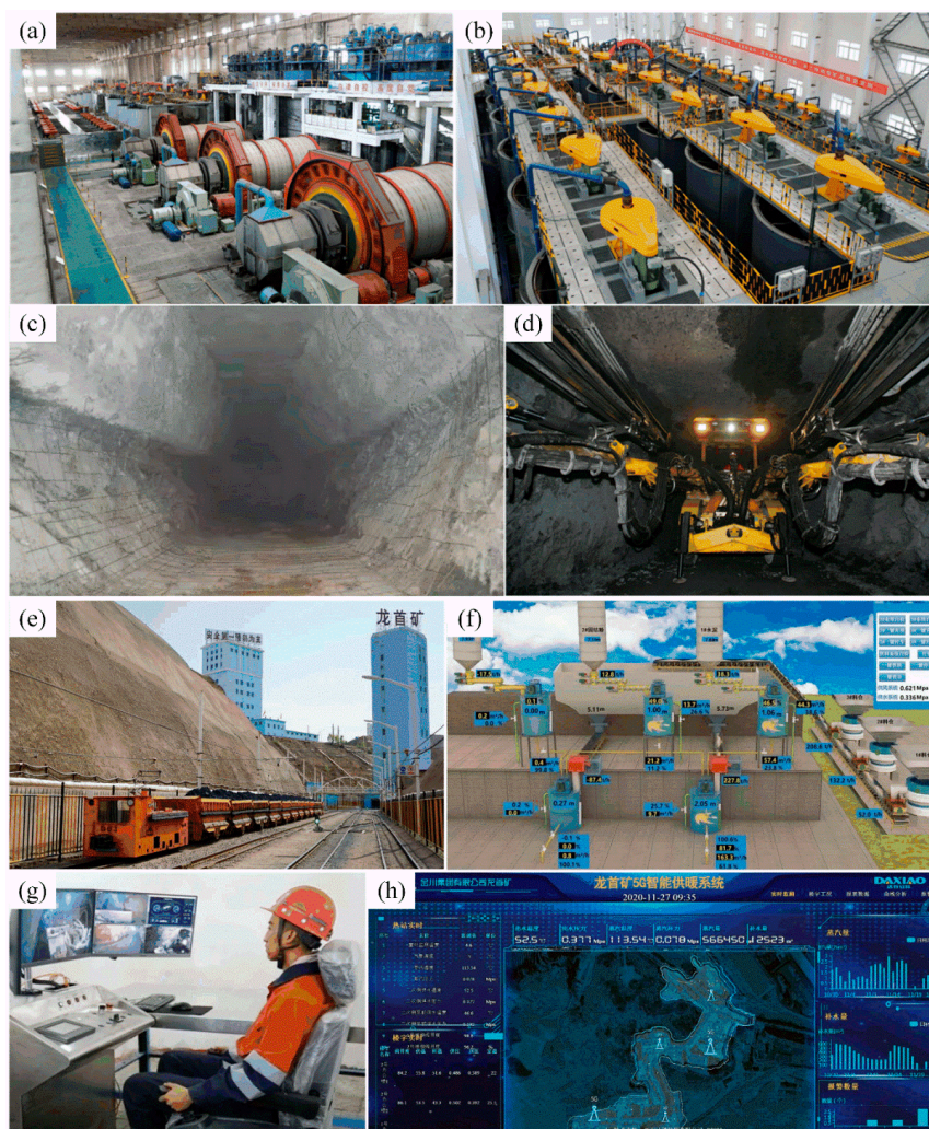
Figure 4. Mechanized and digital management and production systems of Jinchuan Group: (a) ore crushing and ball mill workshop (source from: http://m.stdaily.com/index/kejixinwen/2021-06/19/content_1158139.shtml , access on 15 May 2022); (b) concentrate flotation workshop (source from: https://baijiahao.baidu.com/s?id=1644992078367966371&wfr=spider&for=pc , access on 15 May 2022); (c) downward hexagonal approach (source from: http://www.qzsyg.com/zixun/1/34428248.html , access on 15 May 2022); (d) JCZY-252 wheeled full hydraulic rock drilling rig (source from: https://www.163.com/dy/article/G8015NJ60534697A.html , access on 15 May 2022); (e) 5G+ electric locomotive driverless (source from: https://www.sohu.com/a/440557404_120206435 , access on 15 May 2022); (f) control interface of one-key backfill system in mine (source from: https://www.meipian.cn/3bnpq4hj , access on 15 May 2022); (g) JCCY-6 remote control LHD produced by Jinchuan Group (source from: http://gansu.gansudaily.com.cn/system/2021/04/25/030323276.shtml , access on 15 May 2022); (h) 5G intelligent heating system in mining area (source from: Jinchuan Group).
