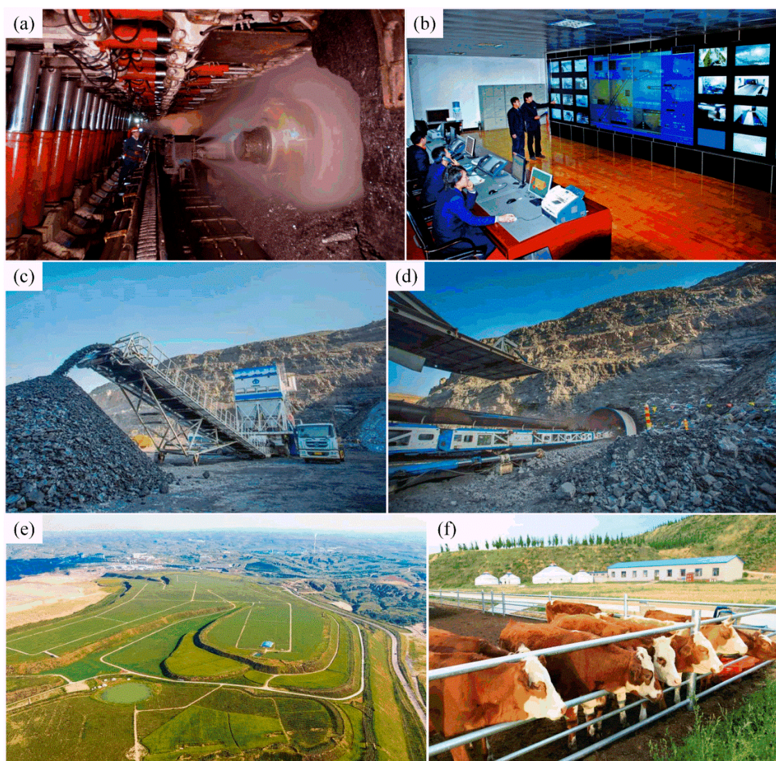
Figure 8. Mining conditions of the Pingshuo Coal Co., Ltd.: (a) fully mechanized mining face (source from: http://xjcec.com/c/2019-10-21/503848.shtml , access on 15 May 2022); (b) surface dispatching control room (source from: Pingshuo Coal Co., Ltd.); (c) edge coal mining system (source from: https://www.sohu.com/a/503659750_121123743 , access on 15 May 2022); (d) border coal transport system (source from: https://www.sohu.com/a/503659750_121123743 , access on 15 May 2022); (e) reclamation of the dump (source from: https://www.sohu.com/a/249352885_160197 , access on 15 May 2022); (f) construction of modern ecological agriculture (source from: https://www.sohu.com/a/249352885_160197 , access on 15 May 2022).
