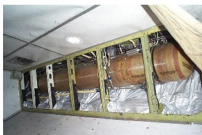
Figure 2. Aircraft potable water tank.
