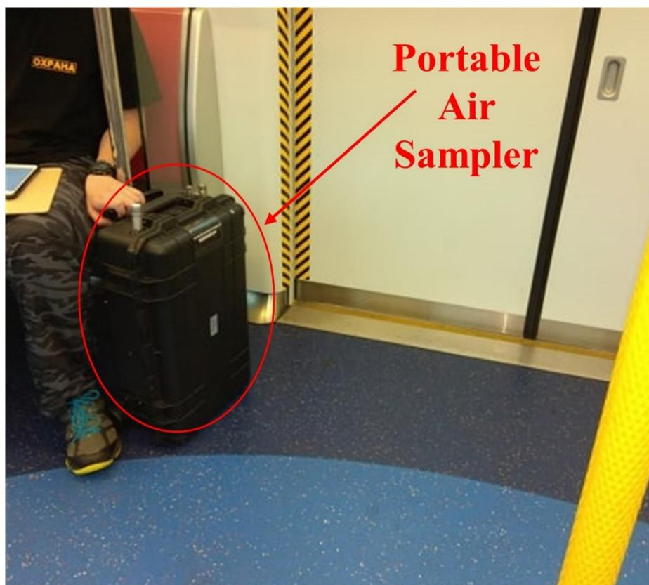
**Figure 1.** Real-time (24 h) personal air quality measurement using portable air sampler.
