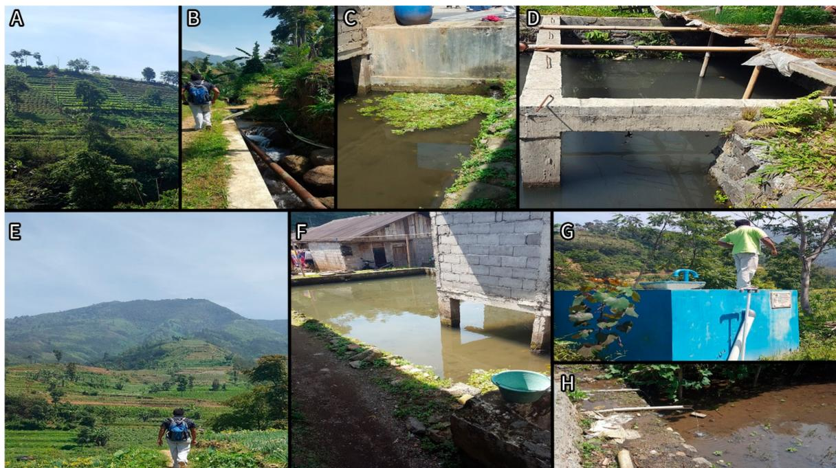
**Figure 4.** Flow of water in Topengan. (A,E)—Surrounding environment of Topengan village. (B)—Pipes from the spring to the holding tank. (C)—Concrete outflow channel to the fishpond. (D)—Crops grown above the fishpond. (F,H)—Fishpond. (G)—Water holding tank.
