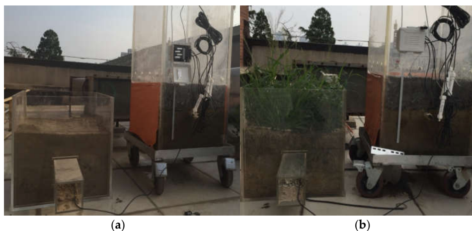
Figure 2. Experimental layout of permeable concrete pavement: (a) control group of bare soil; (b) control group of nature vegetation
