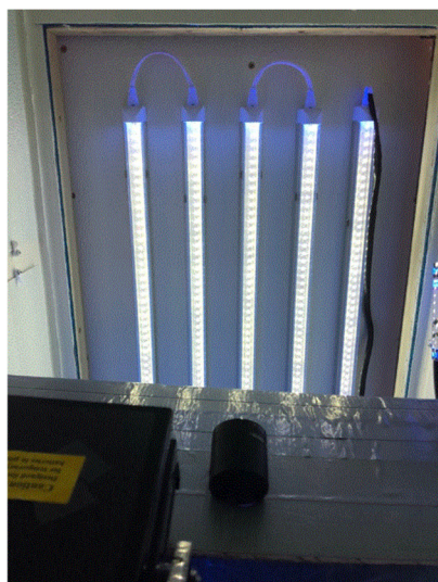
Figure A.3. Picture of measurement of light intensity inside the chamber in the mobile laboratory.
