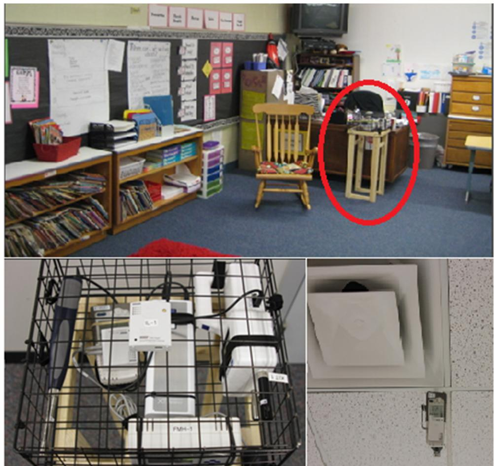
**Figure 1.** Equipment housing placed next to teacher's desk (photo on the top), close looking of the special housing (photo at the lower left), hanging CO<sub>2</sub> m (photo at the lower right) [8].
