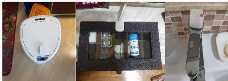
**Figure 5.** Examples of vibration sensor installation (bin, pill organizer, bathroom faucet).
