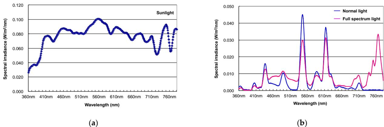
**Figure 1.** Comparison of the spectrum data in (a) sunlight (in September, noon, through the window, exposure value 6500 lx), (b) normal light (blue, color rendition index 81, exposure value 780 lx) and (b) full-spectrum light (magenta, color rendition index 94, exposure value 750 lx). Spectral irradiance of the light spectrum was measured by an illuminance spectrophotometer (CL-500A, Konica Minolta, Inc., Tokyo, Japan).
